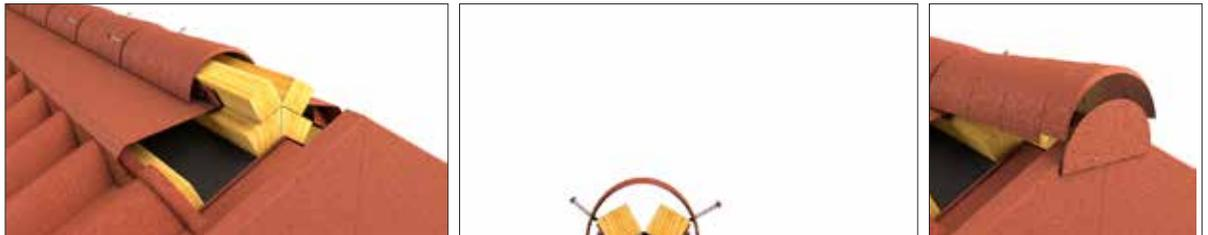
**i** Install the ridge overlaps facing away from prevailing weather.
