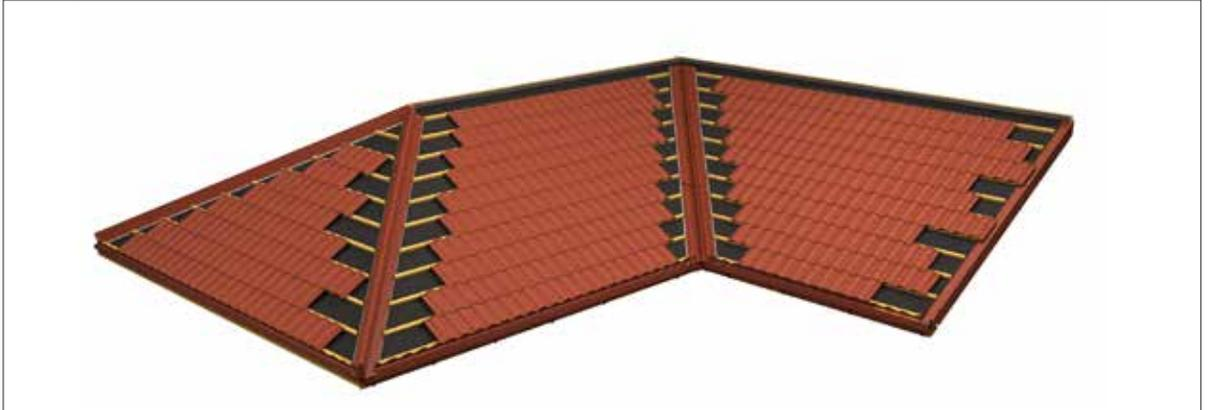
Spanish Barrel is overlapped from left to right. Start at the first full course below the ridge. Lay this course of panels fastening through the back flange into the top of the batten. Do not install full panels tight to the gable, hip, valley, wall or any protrusion such as a skylight or chimney.
