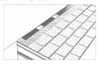
Determine amount of ventilation required and length of slot. Cut a horizontal 1" slot in the deck right before the wall. Leave 6" uncut on each end of the slot. Install underlayment and shingles per
