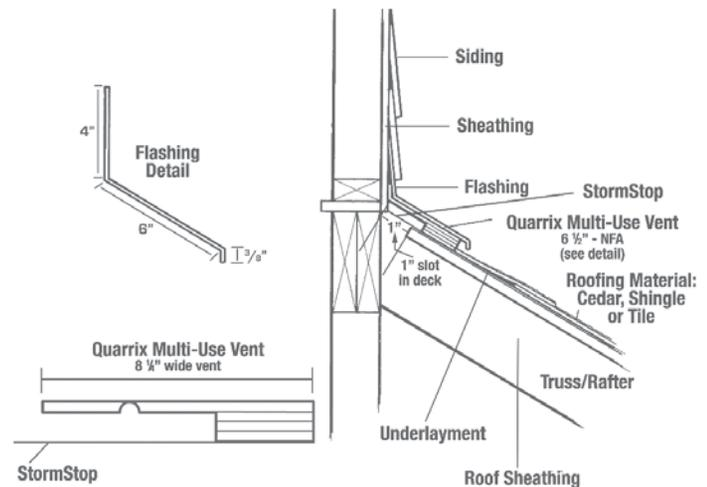
Notes: Install with continuous soffit ventilation at each eave.
