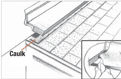
membrane 1/2" by the thick part of vent. Place sealant on both sides of StormStop membrane. Insert foam end cap with the cut-back StormStop
