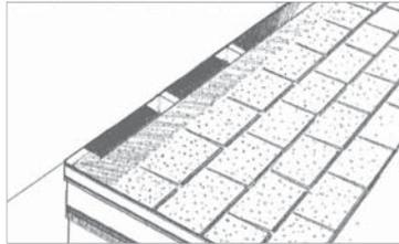
Determine amount of ventilation required and length of slot. Cut a horizontal 1" slot in the deck right before the wall. Leave 6" uncut on each end of the slot. Install underlayment and shingles per manufacturer's instructions. Do not cover pre-cut slot. After field tile installation, the ridge now is ready for vent installation.
