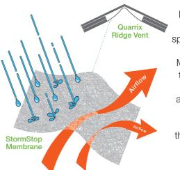
In extreme weather conditions, the spun-bound material of the StormStop Membrane protects the attic and keeps moisture out while allowing continuous airflow. StormStop is engineered so that moisture simply beads up and runs off to protect the attic space.
