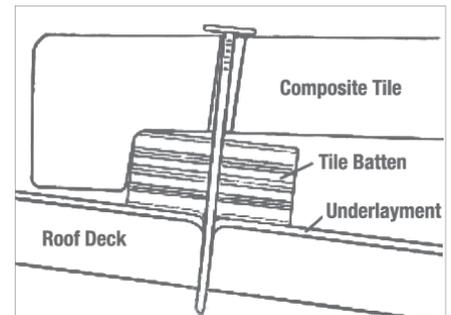
If fasteners are used to secure the tile to the roof, the penetration of the fastener must be into the roof deck for structural hold\* according to the manufacturer's specification.
