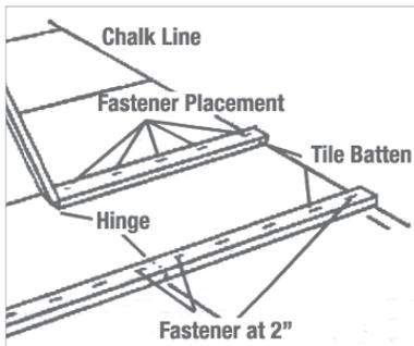
Unfold Quarrix Tile Batten to full 8-foot length and align along pre-chalked line. Nail or staple 2" in from the starting edge. Move over to the hinge of the Tile Batten and nail or staple 2" from hinge of the fold. Note: Power nail or staple tools can be used to place fasteners.
