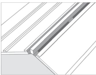
the slot is cut and the battens are installed, it is time to install the field and trim tiles per the tile manufacturer's installation instructions. After field tile installation, the ridge now is ready for vent installation.
