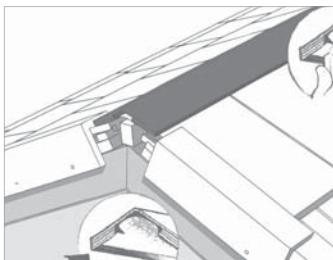
cut back at the end of the vent. Insert the foam end cap with the cut-back StormStop material between the foam end cap and the underside of the vent to assure a weather-tight seal.
