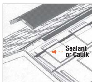
Multiple lengths of vent can be joined by butting the sections tightly together. An end cap should be inserted at the end of each section.
