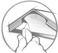
Pull apart a precut section of the foam end cap found with the vent. For products with StormStop, using a utility knife, make a cut in the StormStop material  $\frac{1}{2}$ " on each side, back from the end of the section. Using construction adhesive or sealant caulk, coat both sides
