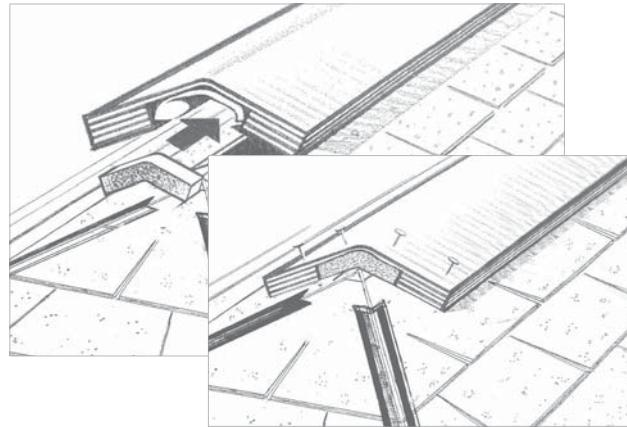
we require that a bead of sealant be applied to the roof shingles before installing the vent on the ridge. This sealant should fill any voids between the bottom of the vent and the surface of the shingle. Use either butyl sealant conforming to ASTM C1085, latex sealant conforming to ASTM C834, silicon sealant complying with ASTM C 920 or asphalt roofing cement complying with ASTM D4586.
