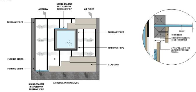
\*If different wood or metal structural furring strips are required along the wall, ProTect Furring Strips can provide valuable wall system support at the top and bottom of the wall to allow proper ventilation of cavity to remove moisture and keep the wall protected and dry.
